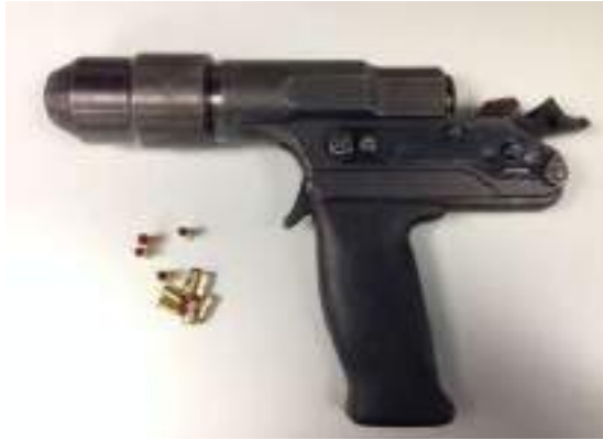
Figure 7.2 A captive bolt pistol with cartridges used to propel the bolt. The apparatus must be well maintained after use.
